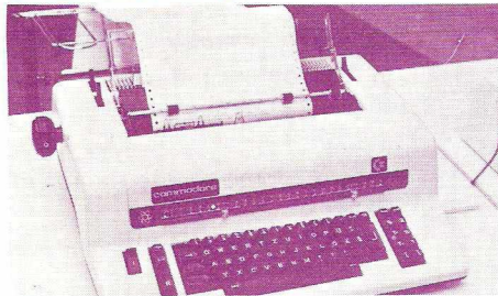
The converted Olympia daisy-wheel typewriter.
